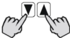
To convert to Celsius units, press the Up and Down buttons simultaneously. Press them again to return to Fahrenheit units.
